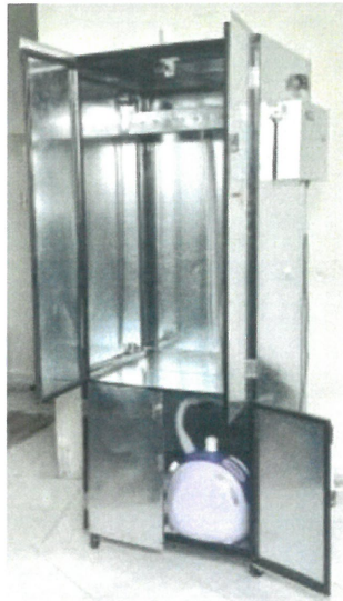
FIGURE 5. Prototype of an automatic cloth ironing machine
