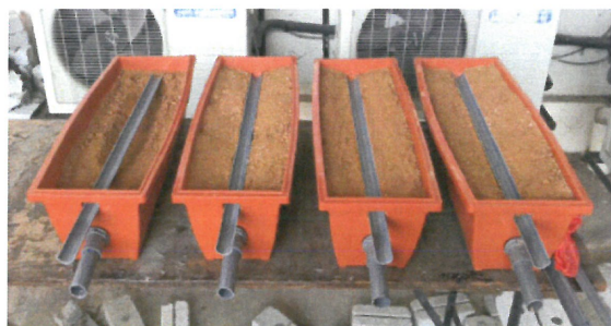
Figure 2. Arrangement of pipe as drainage
