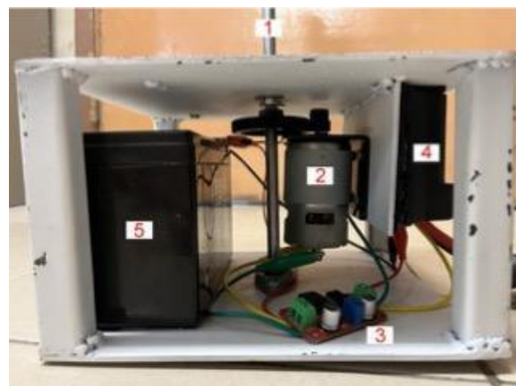
Fig. 8. Side view of frame and components. (1) Shaft connected to VAWT and gears; (2) DC motor; (3) DC-DC Boost Power Module; (4) PWM BCC; (5) 12 V Battery.
