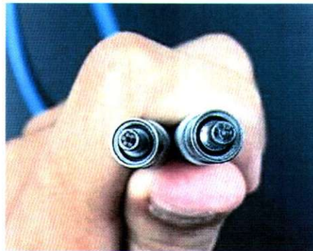
Fig. 2. Cross section of the separate fibre cable leg of Fibre Bundle Probe.
