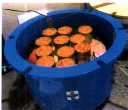
Fig. 3. Plate pressure extractor apparatus.
