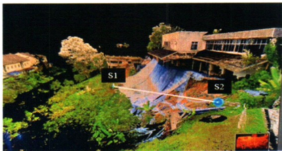
Fig.4 The positions of the TLS at the site. S1 is at the front, and S2 is at the side of the landslide.
