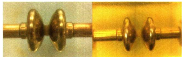
Fig. 7. Cellulose particles' accumulation at 35 kV
