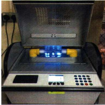
Fig. 3. AC breakdown test instrument for testing liquid dielectric breakdown [9]
