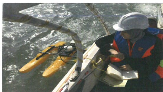
FIGURE 3. Measurement of bed levels, water depths and velocities using the M9 device
