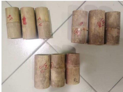
FIGURE 4. Cylindrical shape of bamboo sample for compression test
