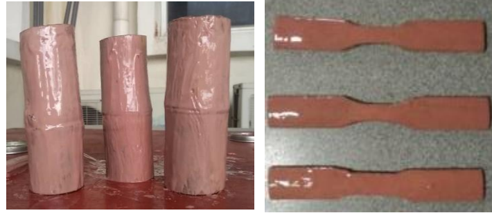
(a) Bamboo coated with solid epoxy
