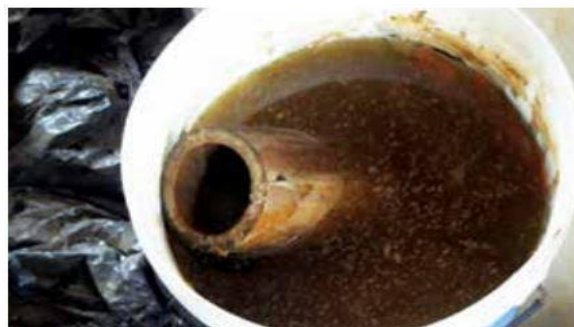
FIGURE 3. Bamboo culm soaked in water
