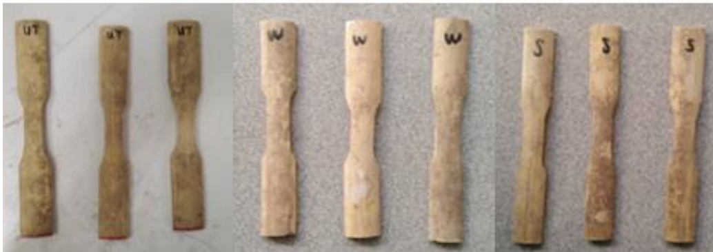
FIGURE 6. Dog-bone shape of bamboo sample for tensile test
