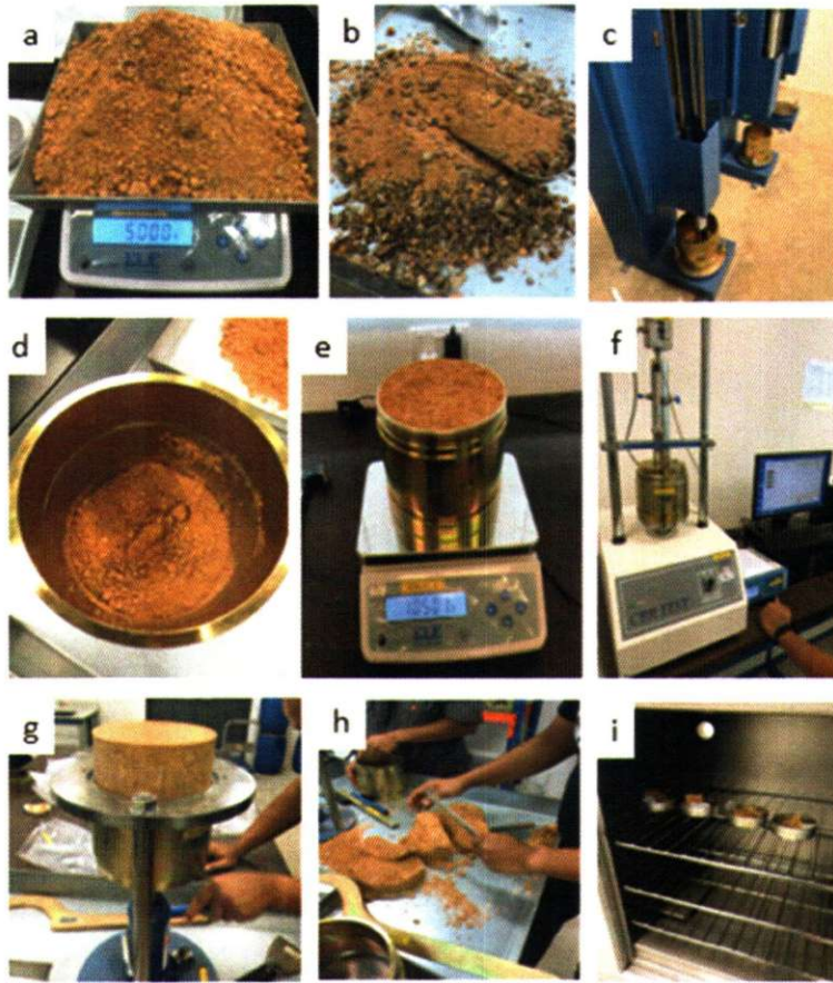
Fig. 4. The CBR test procedures according to MS1056:PART4:2005
