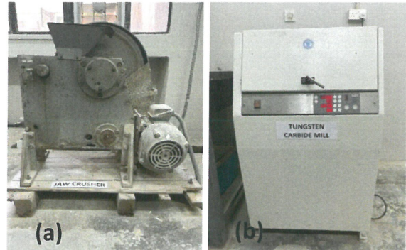
Figure 3. Rock sample preparation using (a) jaw crusher (b) tungsten carbide machine.
