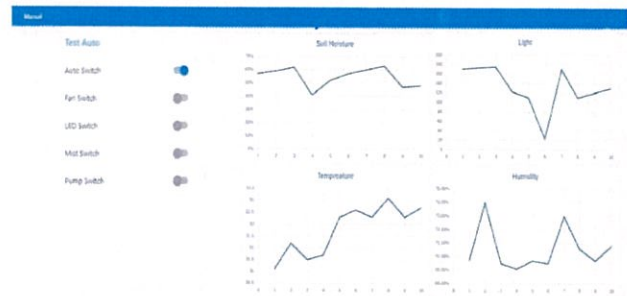
Fig. 13 Node-Red Dashboard including line charts of each environmental factor
