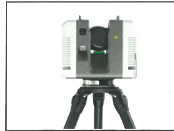
FIGURE 1. Terrestrial Laser Scanner Leica RTC360
