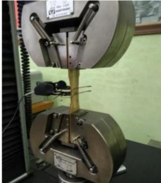
FIGURE 5. Tensile test set up in Universal Testing machine
