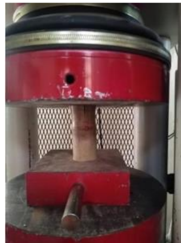
FIGURE 3. Compressive test set up in Compression Testing machine
