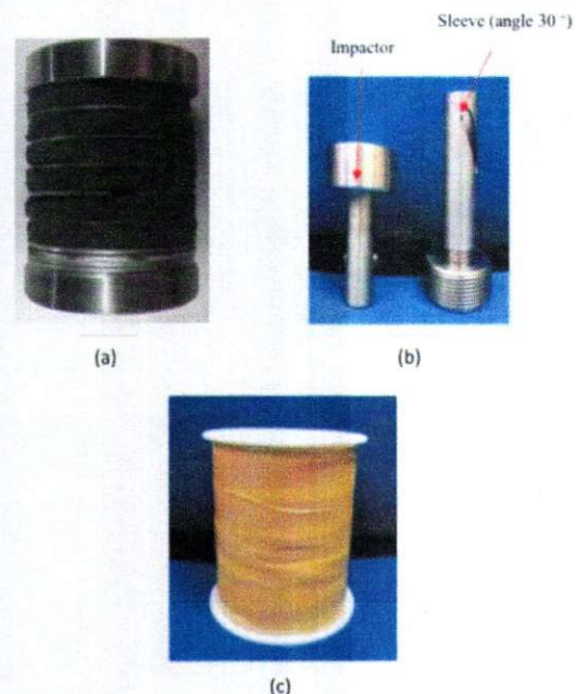
Fig. 4. MRE testing devices (a) MRE isolator device (b) Sleeve and impactor (c) Coil bobbin
