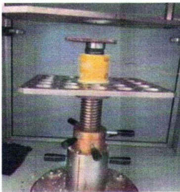
Fig. 6. Configuration MRE device on the impact test rig
