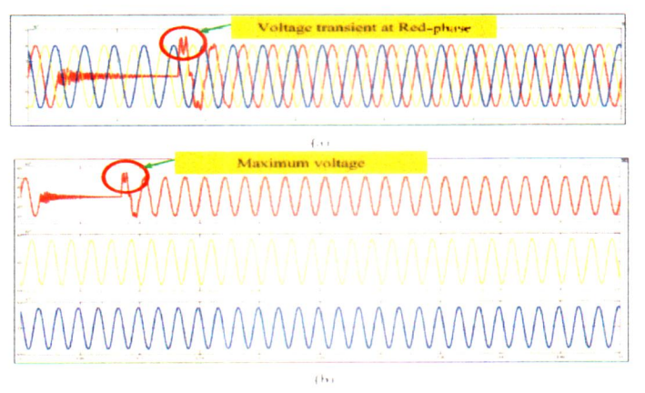
FIGURE 6. (a) Output voltage (b) R – Y – B output
