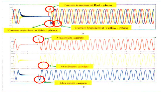
FIGURE 11. (a) Output current (b) R – Y – B output current 3L - G fault.current 3L - G fault.
