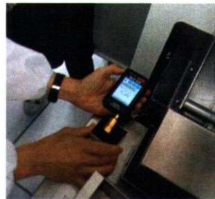
(ii) Measuring static charge of the units after pouring out from the vial
