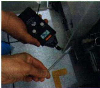
(i) Measuring static charge of the pen
