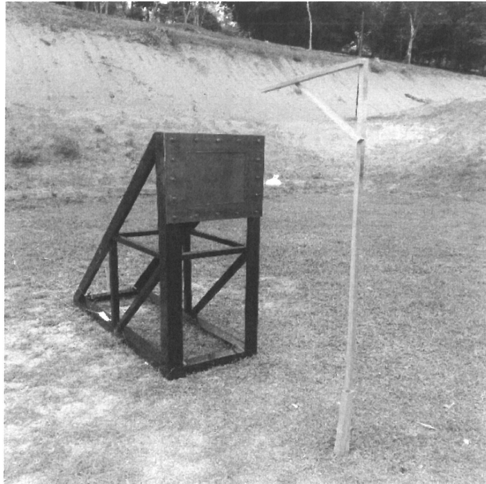
Figure 2: Experimental setup for explosion test Case 1 –Steel Plate only
