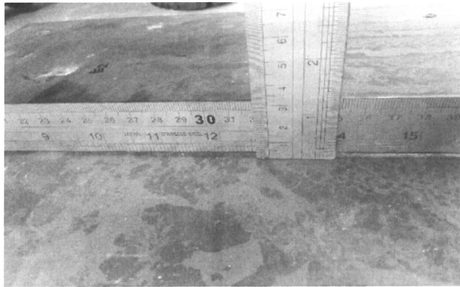
Figure 7: Deflection of steel plate + gypsum
