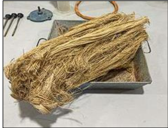
Figure 1. Raw Uncut Bamboo Fiber of Gigantochloa Scortechinii Species
