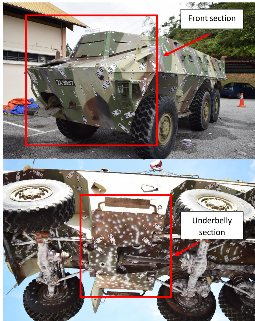
Figure 1.3: Front and underbelly sections of SIBMAS AFSV.
