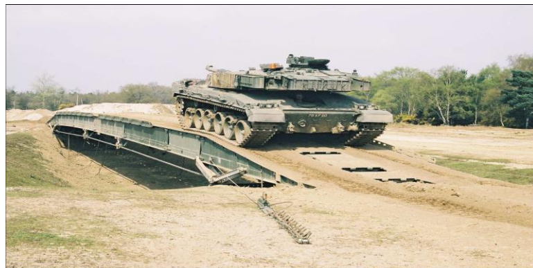
Figure 1.2: Armored vehicle crossing on BR 90 Bridge (Alvis, 2003)
