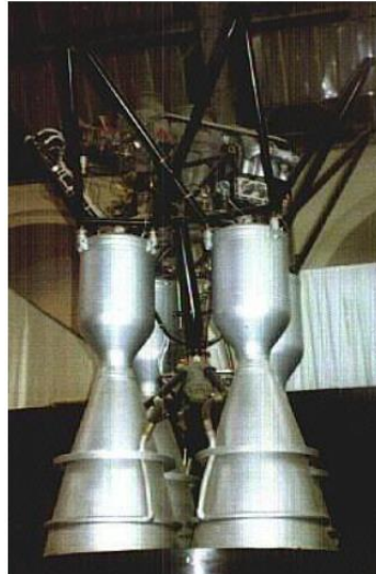
Figure 1.1: Replica of RD-108 LPRE (Wade, 2020)
