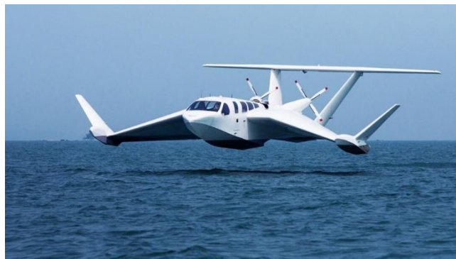
Figure 1.1: A marine craft using WIG phenomenon [1]
