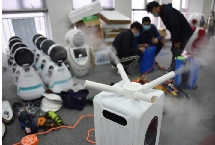
Figure 1.2 A disinfection robot developed to fight against COVID-19 in Qingdao, East China's Shandong province
